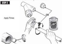
THE MOST FREQUENT CAUSE OF JOINT FAILURE IS INADEQUATE PRIMER PENETRATION. AND SOFTENING OF BONDING SURFACES DURING THE WELDING OPERATION.
